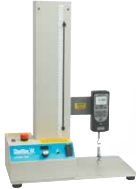
DFS II gauge mounted to LTCM100 tester
